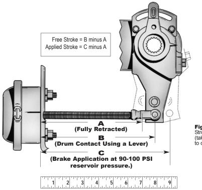
Figure 13 Stroke Measurements (taken from face of air chamber to center of clevis pin)
